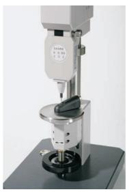
digi test II Shore A, A0, B, C, D, D0, 00, 000, 000 S, micro Shore A micro Shore D, C D0, IRHD/DIDC M, N, H, L, VLRH Normen DIN ISO 7616, DIN EN ISO 868, ASTM D 2240, DIN ISO 48, DIN ISO 27588, NFT 46-003
